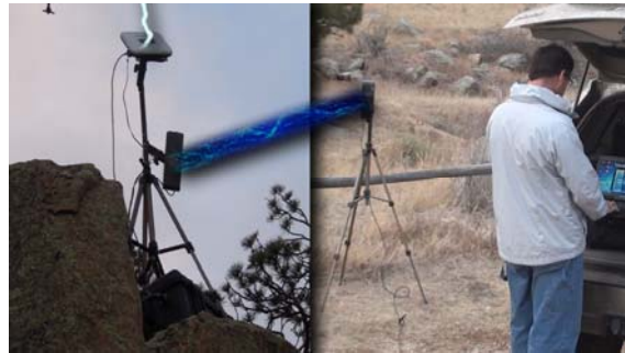
SATPAK Relaying Signal Into BLOS Location
